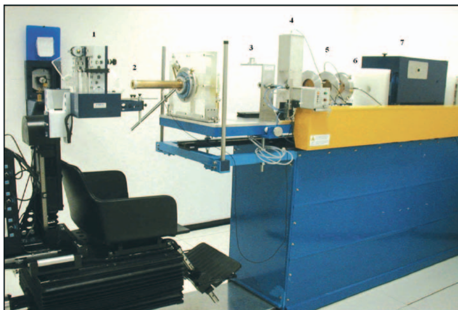
Fig. 1 - View of the CATANA proton therapy facility: 1. Treatment chair for patient immobilization; 2. Final collimator; 3. Positioning laser; 4. Light field simulator; 5. Monitor chambers; 6. Intermediate collimator; 7. Box for the location of modulator wheel and range shifter.
